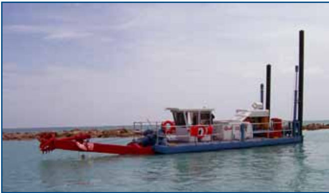
370-20 (6 m) dredging a marina
