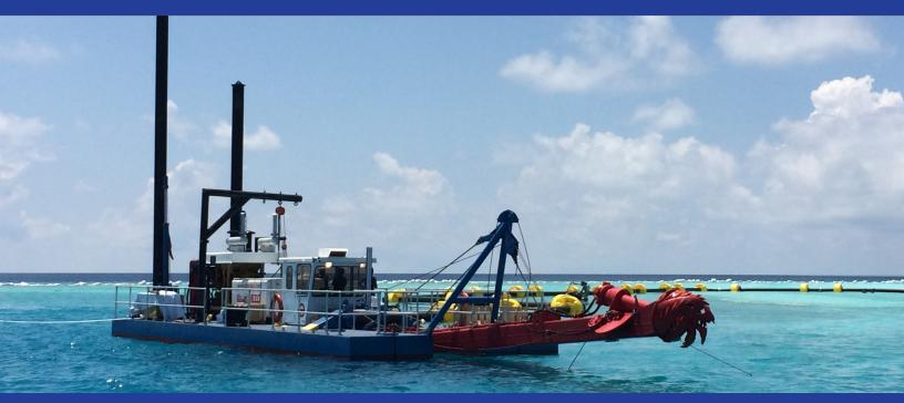
14" x 14" (350 mm x 350 mm) Hydraulic Cutter Suction Dredges
