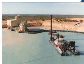
The Cooljarloo , built for mineral mining, one of the world's largest bucketwheel dredges - Australia
