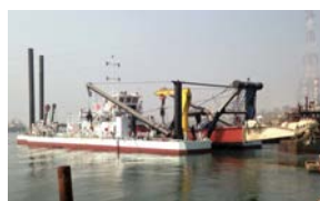
One of four 26" Super Dragon™ dredges built for flood control and navigation projects - Bangladesh
