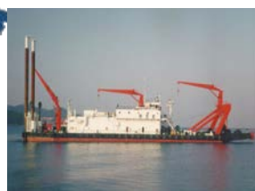
PD-5 , a 17,000 HP (12,700 KW) Super Dragon™ built for a large land reclamation project - South Korea
