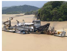
The Mindi, a 10,000 HP, 28" dredge maintaining depth in the Panama Canal - Panama
